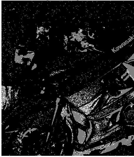
(b) different modes indication on image “bike3”, where grey area indicates run-mode; white dots indicate ternary-mode; dark area indicates regular-mode.
